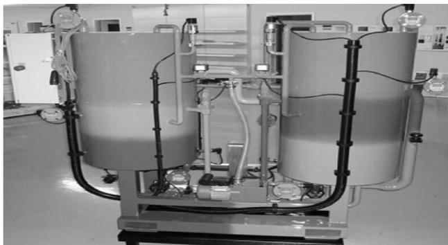
Figure 5: Small size single effect absorption cooling machine
